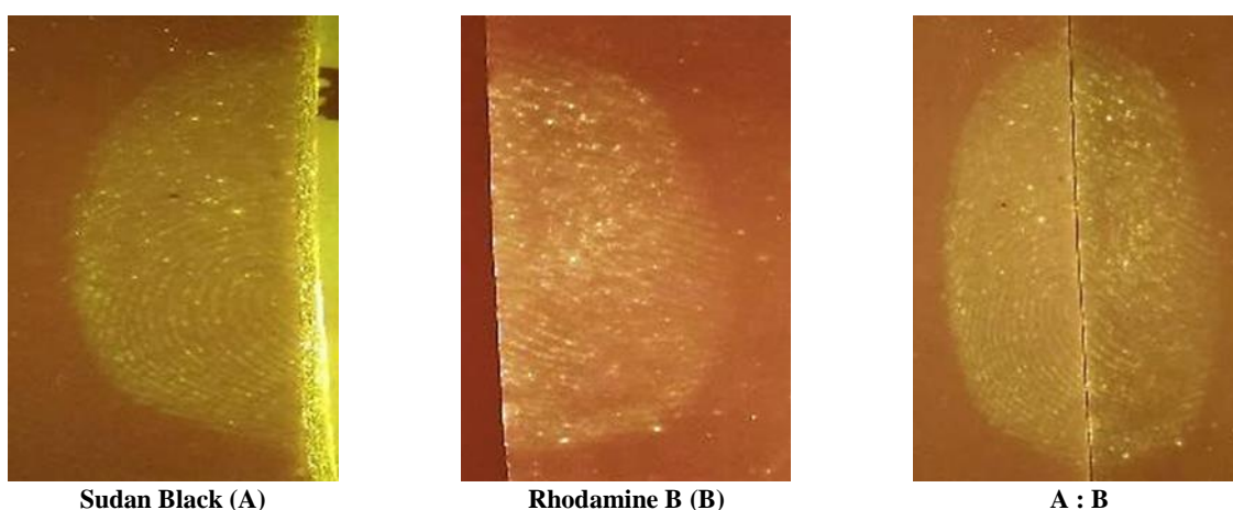
Figure 6: Fingermarks developed on tile substrate in accelerated ageing study
